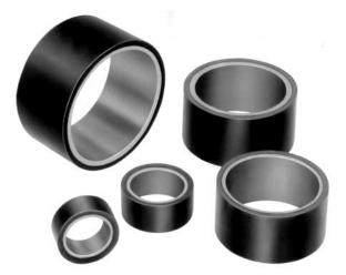
E&E urethane tires are used to protect and silence cam followers in applications where metal to metal contact is objectionable. The resilient tires cushion impact and reduce wear, extending follower life. They also prevent marring of finished surfaces. E&E urethane tires are available in a variety of sizes to pressfit over standard cam followers.
